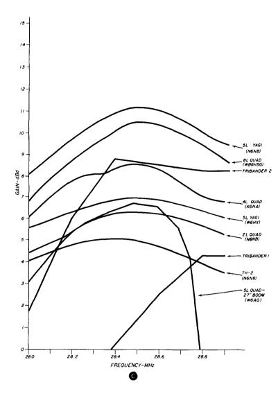
All of my antennas were experimentally optimized that way. One can derive good element spacings and lengths, and scale those values to lower frequencies, as long as frequency-related variables such as changing length-to-diameter ratios are not overlooked.
